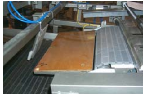
Gravity Lid Pick-Off and Insert Conveyors
