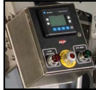
Machine Mounted Operator Control Station
