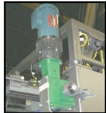
Main Carriage Drive
