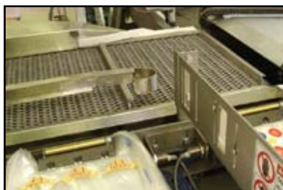
Flusher Discharge Conveyor
