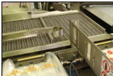
Flusher Discharge Conveyor
