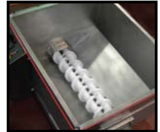
Twin Screw Auger Design
